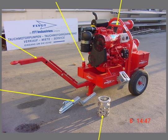
Accessory (FA production): Stainless steel suction strainer incl. 4"-coupling part (Storz)
