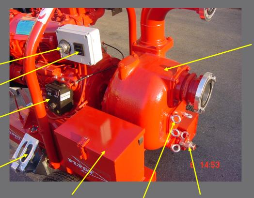
Special pump housing with bigger impeller troughlet (45 mm)
