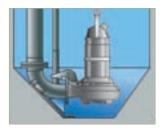
The small floor and optimised geometries ensure high water velocity that whips settled solids into suspension.
