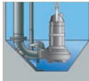
The TOP sump design with integrated discharge connection. Its sloping sides result in high flow velocities, creating turbulence that re-suspends solids, dramatically improving solids transport.
